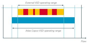
Flow gaps due to vibration and noise issues
