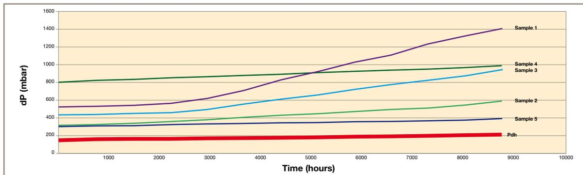
Test criteria: Filters were tested at their full rated flow and injected with ISO 12103 A4 course test dust using a pressurized dust injection system. The dust was injected in 12 intervals to simulate the monthly loading of the filter element and show a total annual differential pressure curve. OIL-X EVOLUTION filters were tested at an identical flow rate to the comparative filter and with an identical dirt loading.
